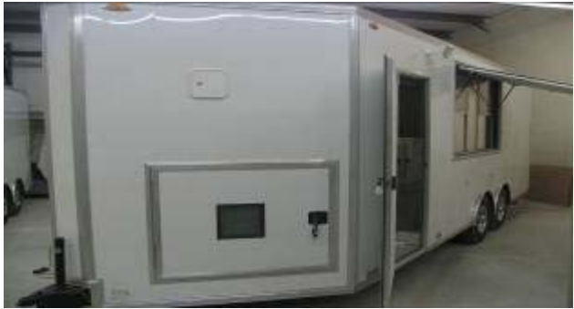
Below: The outside showing the serving window access doors. The small door on the front V nose houses the installed 12kw diesel generator.
